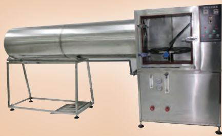
強衝水試驗箱 (Flush Test Chamber) 用於檢驗產品的密封、防水性能 Test the sealing, waterproof performance of products
