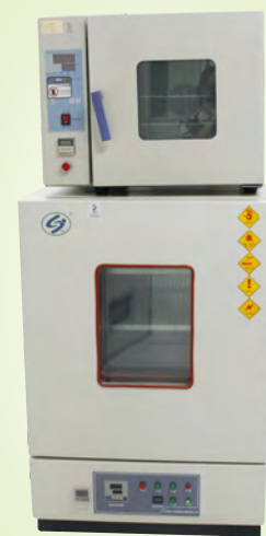
高溫烤箱 (Flush Test Chamber) 模擬產品耐受高溫儲存，評估產品外觀及功能變化狀況 Simulate products' tolerance in high temperature and assess the changes in appearance and function
